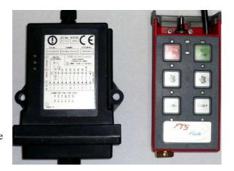
A LED displays whether there is a radio connection or not. Automatic or manual frequency-switching between 3 channels
